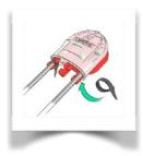
The TRT-300 A acts as a remote contact interface that can activate or deactivate a third party instrument or equipment that needs to be triggered during a live-broadcast of an evacuation event. The TRT-300 A sits in the LOOP and receives the broadcast audio message. As soon as the broadcast audio message contains a 20kHz pilote-tone, the on-board relays of the TRT-300 A will change state into 'override' mode. The state change is latched as long as the pilote-tone is received.
