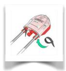
The TRT-400 A is a T-branch field-isolator-module with integrated volume control for the T-branch speaker load. A pilot-tone send over the speaker line will force the TRT-400 A into 'override' mode forcing the attached volume control to switch to maximum audio level. Any local music source connected to the TRT-400 A through the AUX input will mute.
