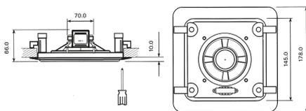
The square cut for the installation should have a side length of 145 mm.
