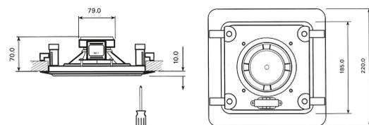
The square cut for the installation should have a side length of 185 mm.
