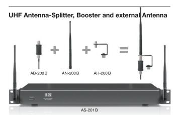
Multi-channel-systems can be assembled with accessory components. The splitter AS-200 B (19″, 1 RU) manages up to 4 transmitters UWR-701 F. The booster AB-200 B provides sufficient amplification (+9dB) as an external cable driver
